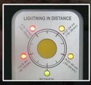
LED Display shows how far away lightning is striking and if storm is approaching or leaving.
