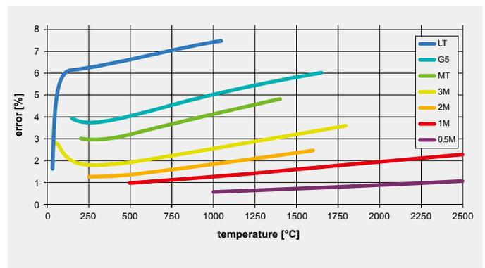
Measurement error of 10 % as result of wrongly adjusted emissivity and in dependence on wavelength and object temperature (LT: 8–14  $\mu\text{m}$ ; G5: 5  $\mu\text{m}$ ; MT: 3.9  $\mu\text{m}$ ; 3M: 2.3  $\mu\text{m}$ ; 2M: 1.6  $\mu\text{m}$ ; 1M: 1.0  $\mu\text{m}$ ); 0.5M: 525 nm.
